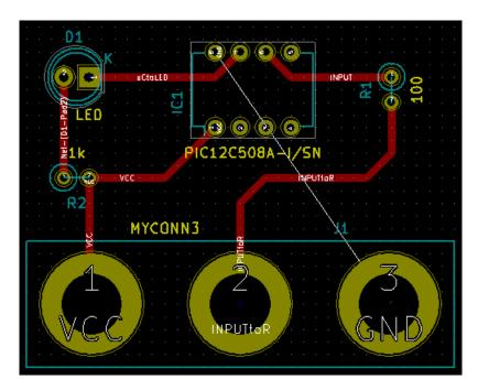
20. Let's now run a track on the other copper side of the PCB. Select *B.Cu* in the drop-down menu on the top toolbar. Click on the *Route tracks* icon. Draw a track between pin 3 of J1 and pin 8 of U1. This is actually not necessary since we could do this with the ground plane. Notice how the colour of the track has changed.
