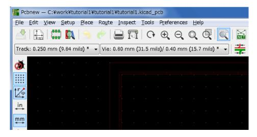
16. If you would like to add more track widths go to: **Setup** → **Design Rules** → **Global Design Rules** tab and at the bottom right of this window add any other width you would like to have available. You can then choose the widths of the track from the drop-down menu while you lay out your board. See the example below (inches).
