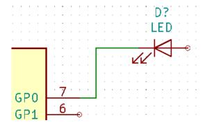
33. Repeat this process and wire up all the other components as shown below. To terminate a wire just double-click. When wiring up the VCC and GND symbols, the wire should touch the bottom of the VCC symbol and the middle top of the GND symbol. See the screenshot below.
